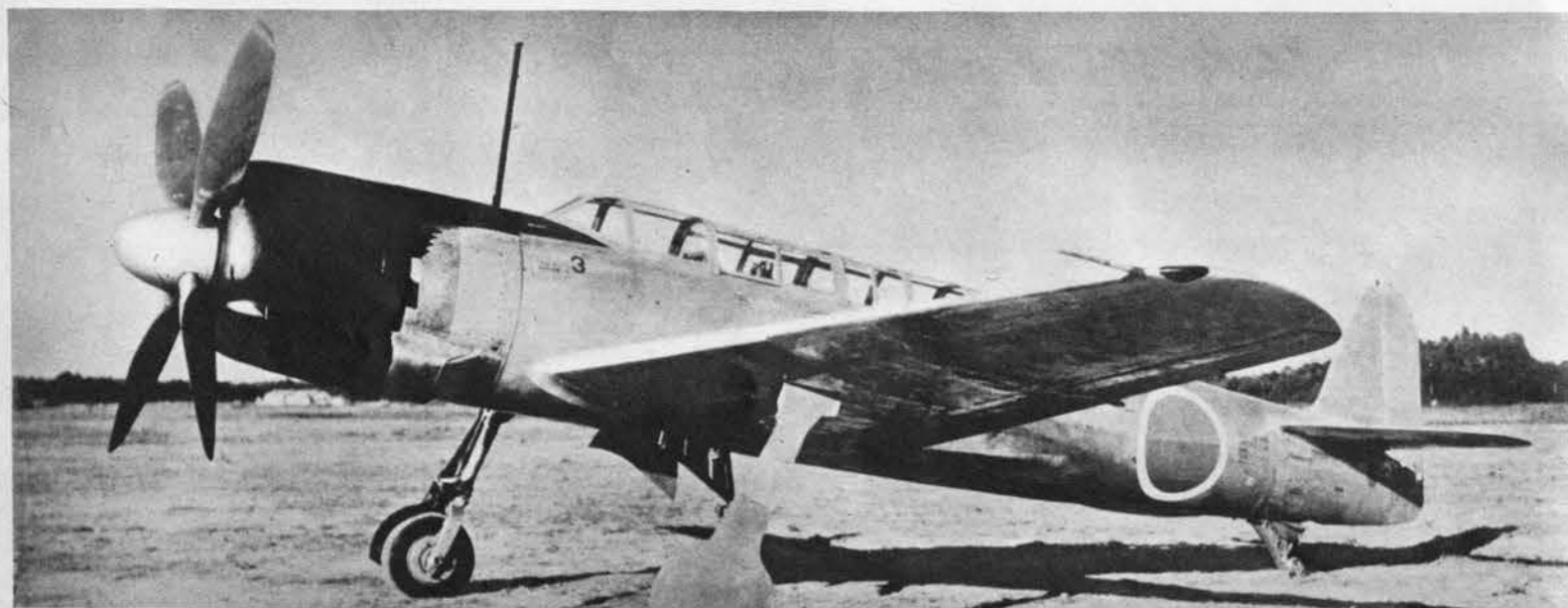
MYRT Carrier-based, Myrt is nearly as fast as Dinah ( above ), has a range of 2,500 miles. It can be recognized by the long greenhouse, exceptionally long nose and the forward lean of fin
